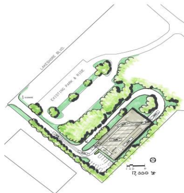
The 2 sketches to left are Conceptual studies prepared for the Laketrans system. There were 5 different building layouts for 10 bus storage showing the least expensive (also least efficient), designs that used all interior bus circulation to those that allowed each bus to have multiple drive through doors.
