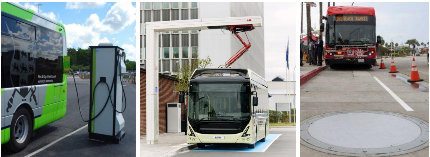
Figure 2-1. Battery Electric Bus Charging Methods
