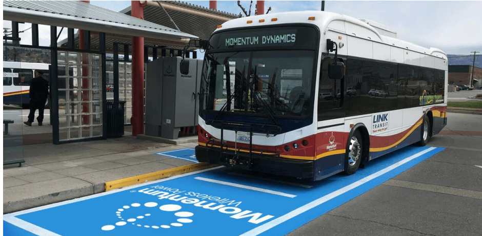
Figure 2-6. On-Route Induction Charging, Link Transit, Wenatchee, Washington
