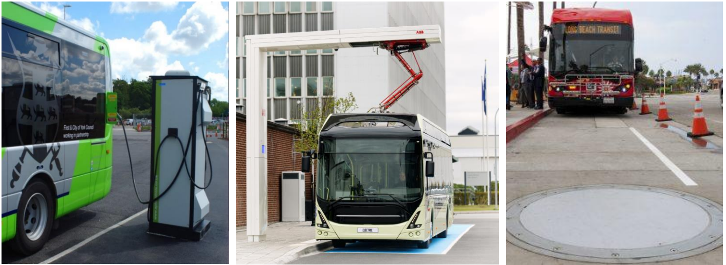
Figure E-1. Battery-Electric Bus Charging Methods
