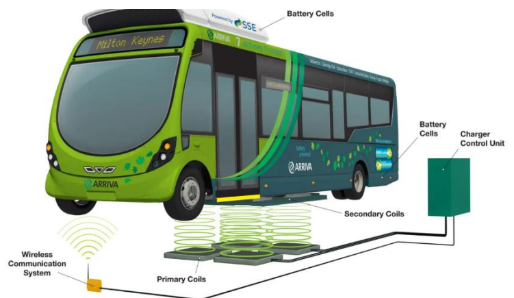
Figure 2-5. Induction Charging Process
